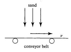
The minimum power required to keep the conveyor belt moving at constant speed while the sand is falling on it will be
