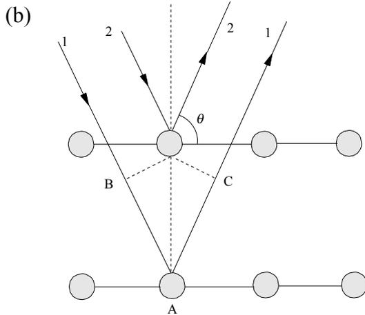
diagram should show two rays one scattered from one plane [1]
