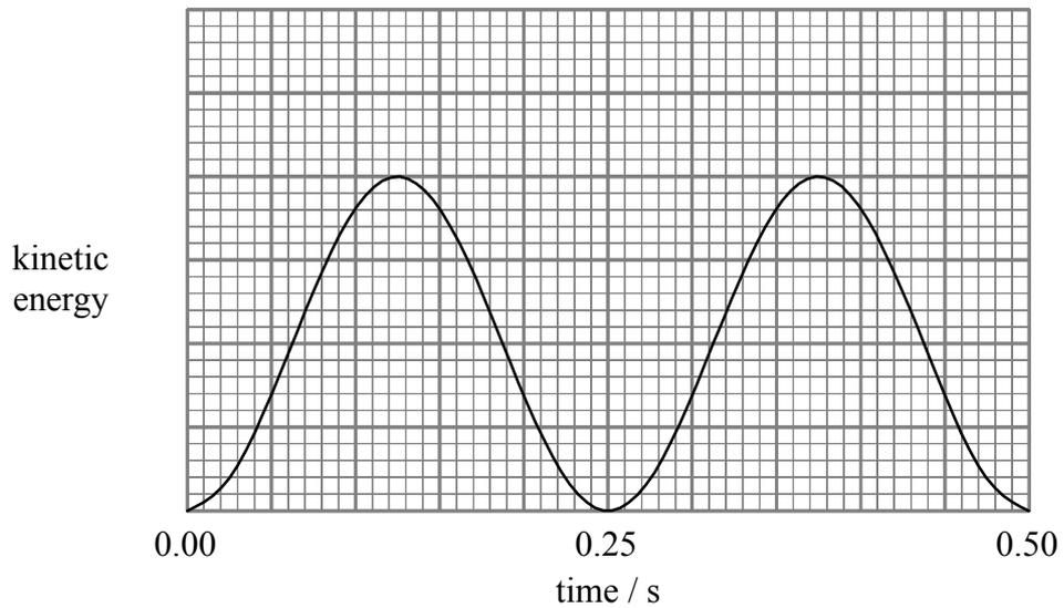
One cycle of a  $\sin^2$  graph or  $\cos^2$  graph with zero for KE marked correct position with respect to the x-axis scale
