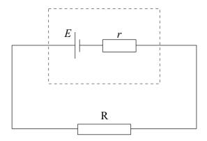
The cell supplies  $8.1 \times 10^3$  J of energy when  $5.8 \times 10^3$  C of charge moves completely round the circuit. The current in the circuit is constant.
