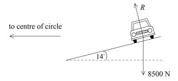
At one particular speed v of the car, there is no frictional force at  $90^{\circ}$  to the direction of travel of the car between the tyres and the road surface. The reaction force of the road on the car is R.
