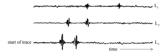
On each record, one pulse is made by the S wave and the other by the P wave. The separation of the two pulses is referred to as the S-P interval.
