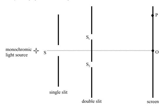
$S_1$  and  $S_2$  are two very narrow slits. The single slit S ensures that the light leaving the slits  $S_1$  and  $S_2$  is coherent.
