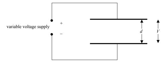
The charge Q on one of the plates is measured for different values of the potential difference V applied between the plates. The values obtained are shown in the table below. The uncertainty in the value of V is not significant but the uncertainty in Q is  $\pm 10\%$ .
