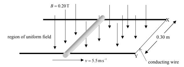
The distance between the rails, X and Y is 0.30 m, the magnetic field strength is 0.20 T and the speed v of the rod is  $5.5 \,\mathrm{m\,s^{-1}}$ .
