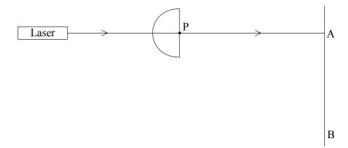
The semi-circular block is rotated about the point P. The spot of light on the screen is seen to move downwards. When the spot reaches point B, it disappears.
