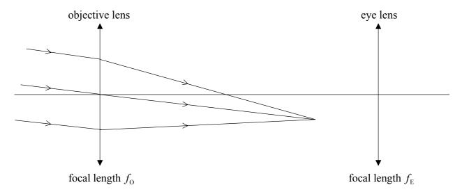
The focal lengths of the objective lens and of the eye lens are  $f_0$  and  $f_E$  respectively. Light from a distant object is shown focused in the focal plane of the objective lens. The final image is to be formed at infinity.
