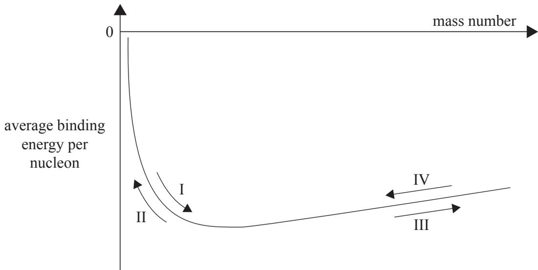
Which direction indicates a fission reaction with a release of energy?
