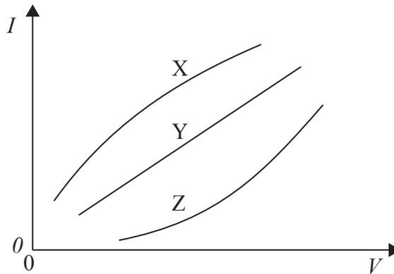
Which of the following corresponds to resistors for which the resistance increases with increasing current?
