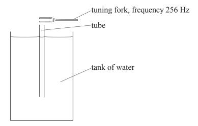
A tuning fork of frequency 256 Hz is sounded continuously above the tube. The tube is slowly raised out of the water and, at one position of the tube, a maximum loudness of sound is heard.
