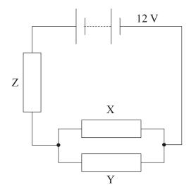
The cell has e.m.f. 12 V and negligible internal resistance. The resistor Z has resistance *R* and the potential difference across the conductors X and Y is 5.0 V.
