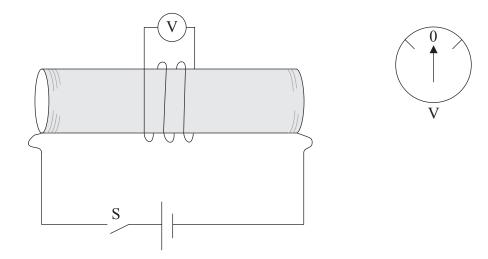
The ends of the wire are connected to a high resistance voltmeter V that has a centre zero scale (as shown in the inset diagram).
