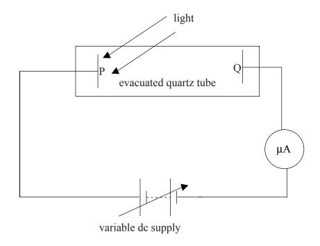
P and Q are metal plates. Monochromatic light of frequency f is incident on plate P. In the situation shown, the microammeter ( $\mu A$ ) registers a current. The intensity of the light is kept constant throughout the experiment.
