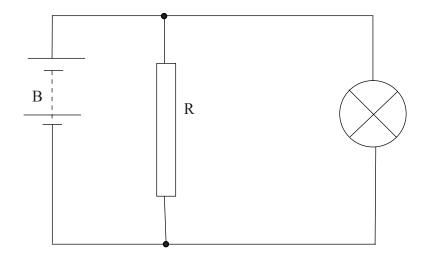
The battery B has an internal resistance of 5.0  $\Omega$  and the resistance R of the resistor is 15  $\Omega$ .
