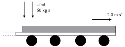
The conveyor belt that is driven by an engine, moves with speed  $2.0 \text{ m s}^{-1}$ .
