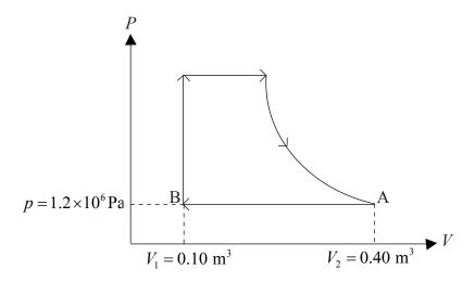
The part of the cycle labelled AB is an isobaric isothermal change of phase.
