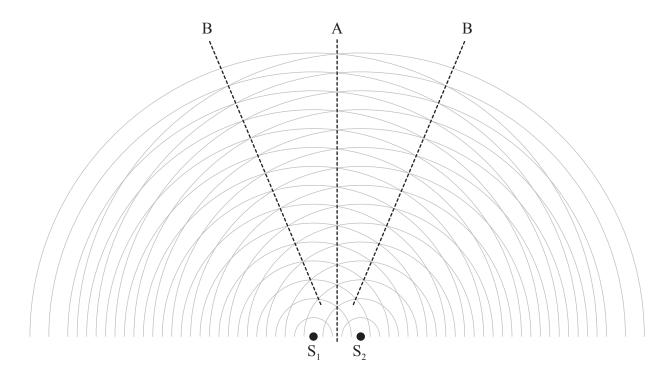
The waves interfere constructively along the lines labelled A and B.
