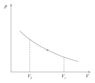
On the diagram above, draw a line to show the variation of pressure p as the volume of the gas is changed from  $V_1$  to  $V_2$  without allowing any thermal energy to enter or leave the gas.
