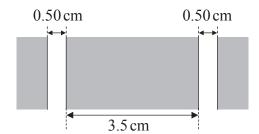
A beam of sound, incident normally to the plane of the double slit, passes through the slits. A detector is moved along a line parallel to the plane of the double slit at a distance of 1.5 m from the slits. The distance between points of maximum sound intensity is 1.2 m. Determine the wavelength of the sound wave.
