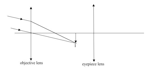
The objective lens has a focal length  $f_{\rm o}$  and the eyepiece lens has a focal length  $f_{\rm e}$ . The objective lens forms an image of a distant object at I. The final image is formed at infinity.
