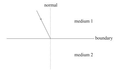
The refractive index of medium 1 is  $n_1$  and that of medium 2 is  $n_2$  and  $n_1 > n_2$ . The ray is incident at an angle to the normal that is less than the critical angle.
