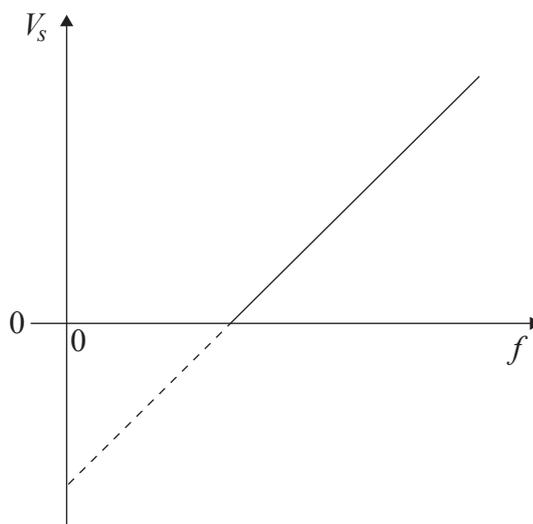
Planck's constant may be determined from the charge of an electron  $e$  multiplied by
