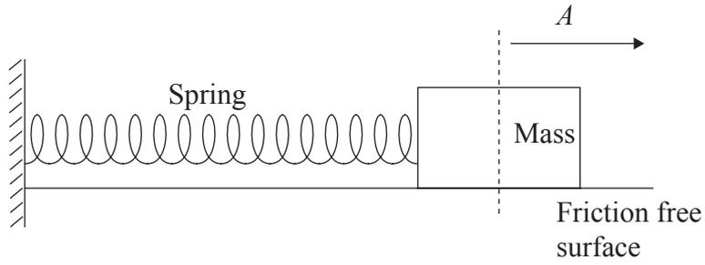
An identical mass is attached to an identical spring. The maximum displacement is  $2A$ . Assuming this spring obeys Hooke's law, which of the following gives the correct time period and total energy?
