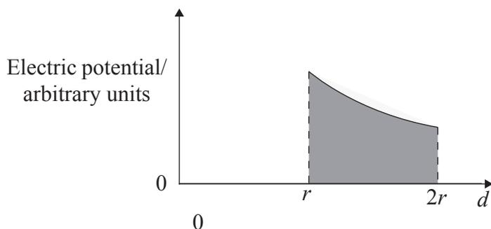
The work done by an external force in moving a test charge  $+q$  from  $d = 2r$  to  $d = r$  is equal to  $q$  multiplied by the
