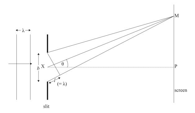
The width of the slit is b and the point X is at the centre of the slit. The point M on the screen is the position of the first minimum of the diffraction pattern formed on the screen. The path difference between light from the top edge of the slit and light from the bottom edge of the slit is l.
