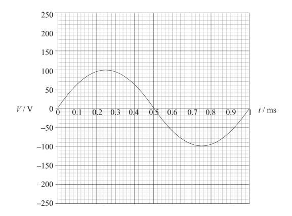
A resistor of resistance 25  $\Omega$  is connected across the output of the generator.
