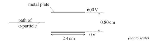
The metal plates are of length 2.4 cm and their separation is 0.80 cm. The potential difference between the plates is 600 V. The electric field is uniform in the region between the plates and is zero outside this region.
