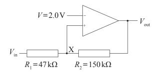
In the situation shown, the potential at point X is  $2.0\,\mathrm{V}$  and the output potential  $V_\mathrm{out}$  is at its minimum value of  $-10\,\mathrm{V}$ . Show that for the output potential to switch to its maximum value of +10V
