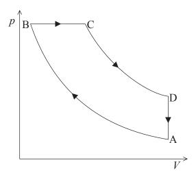
AB and CD are adiabatic changes of state. The pressure at point B is  $1.8 \times 10^5$  Pa and the change in volume of the gas between B and C is  $4.8 \times 10^{-4}$  m<sup>3</sup>.
