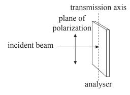
The angle between the transmission axis of the analyser and the plane of polarization of the light is  $\theta$ . In the position shown the transmission axis of the analyser is parallel to the plane of polarization of the light ( $\theta$ =0).
