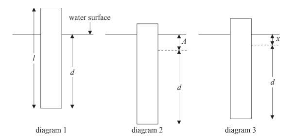
The length of wood below the surface is d. The wood is pushed vertically downwards a distance A such that a length of wood is still above the water surface as shown in diagram 2. The wood is then released and oscillates vertically. At the instant shown in diagram 3, the wood is moving downwards and the length of wood beneath the surface is d+x.
