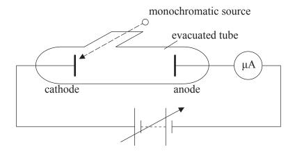
Light from the monochromatic source is incident on a cathode placed in an evacuated tube. A variable voltage supply is connected between anode and cathode and the photoelectric current is registered by the microammeter. The sketch graph shows how the photoelectric current I varies with the potential difference V between anode and cathode for two sources of light, A and B, of different frequencies and intensities.
