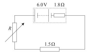
Estimate the resistance R of the variable resistor that will limit the current to  $0.82\,\mathrm{A}$ .
