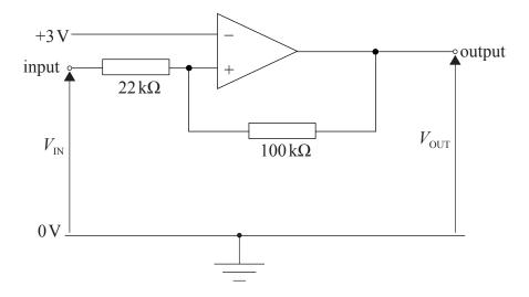
The output of this Schmitt trigger is positive saturation (+13 V) or negative saturation (-13 V).
