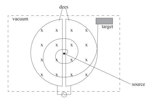
Charged particles are emitted from a source at the centre. They move in a vacuum through two D-shaped cavities or "dees". There is a uniform magnetic field directed into the page, within the region of the dees.
