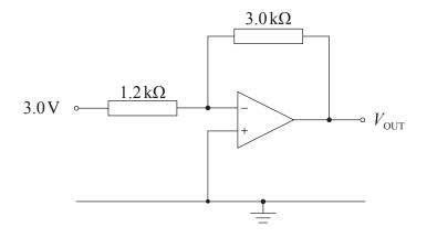
Calculate the output voltage  $V_{\mathrm{OUT}}$ .
