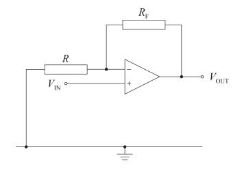
Show that the gain of this amplifier is given by  $G = 1 + \frac{R_F}{R}$ . [3]
