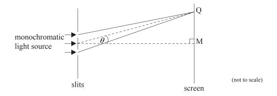
The separation of the slits is large compared to their width. A pattern of light and dark fringes is observed on the screen.
