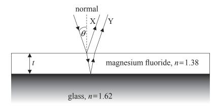
X is a ray reflected from the surface of the film and Y is reflected from the surface of the glass.
