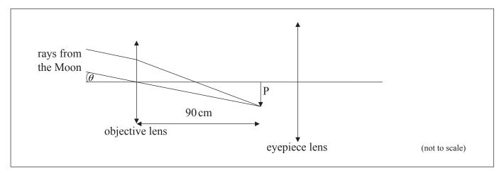
The telescope is in normal adjustment.
