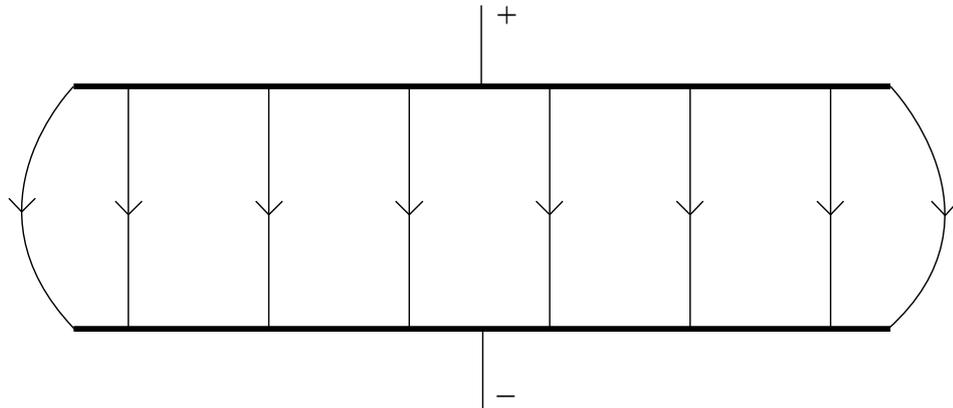
uniform (by eye) line spacing and edge effect, field lines touching both plates;
