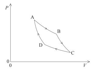
The changes of state from A to B and C to D are isothermal whereas the changes of state from B to C and D to A are adiabatic.
