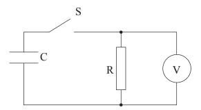
The initial potential difference across C was 12 V. The switch S was closed and the potential difference V across R was measured at various times t. The data collected, along with error bars, are shown plotted below.
