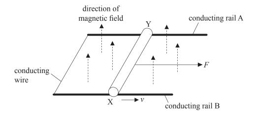
In the situation shown, the rod is moved along the rails at a constant speed v by a constant horizontal force of magnitude F.
