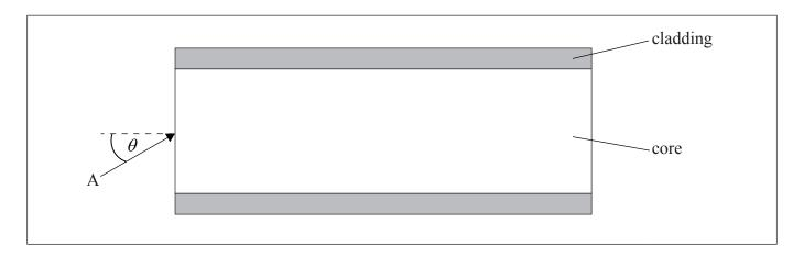
The refractive index of the core is 1.62 and the refractive index of the cladding is 1.52. The critical angle at the core-cladding boundary is  $70^{\circ}$ .
