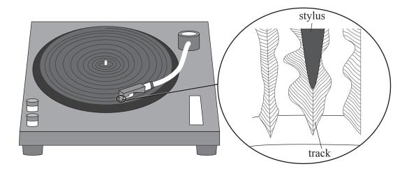
As the LP record rotates, the stylus moves because of changes in the width and position of the track. These movements are converted into sound waves by an electrical system and a loudspeaker.
