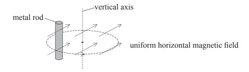
The metal rod completes one circle of radius  $0.060\,\mathrm{m}$  in  $0.020\,\mathrm{s}$  in the magnetic field of strength  $61\,\mathrm{mT}$ .
