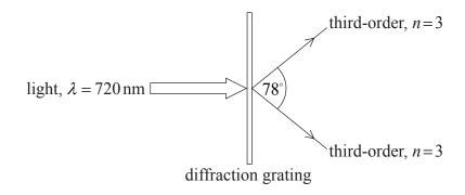
Determine the number of lines per metre of the diffraction grating.
