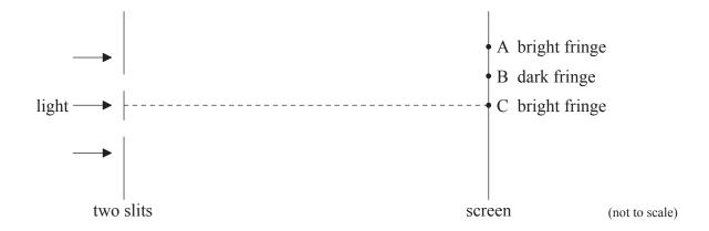
A central bright fringe is produced at C. The next bright fringe is produced at A. There is a dark fringe at B.
