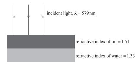
(a) Determine the minimum thickness of the oil layer that gives rise to the least amount of light being reflected.
