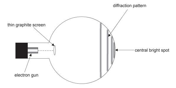
A pattern forms when diffracted electrons are incident on a fluorescent layer at the end of the tube.
