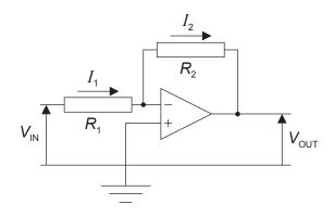
Show that the gain of the amplifier is  $\frac{V_{\text{OUT}}}{V_{\text{IN}}} = -\frac{R_2}{R_1}$ . [3]
