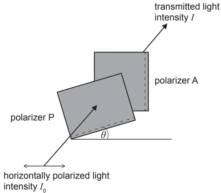
The angle  $\theta$  is varied from 0 to 90 degrees. Which of the following represents the variation with  $\theta$  of the intensity  $I$  of the light transmitted through A?
