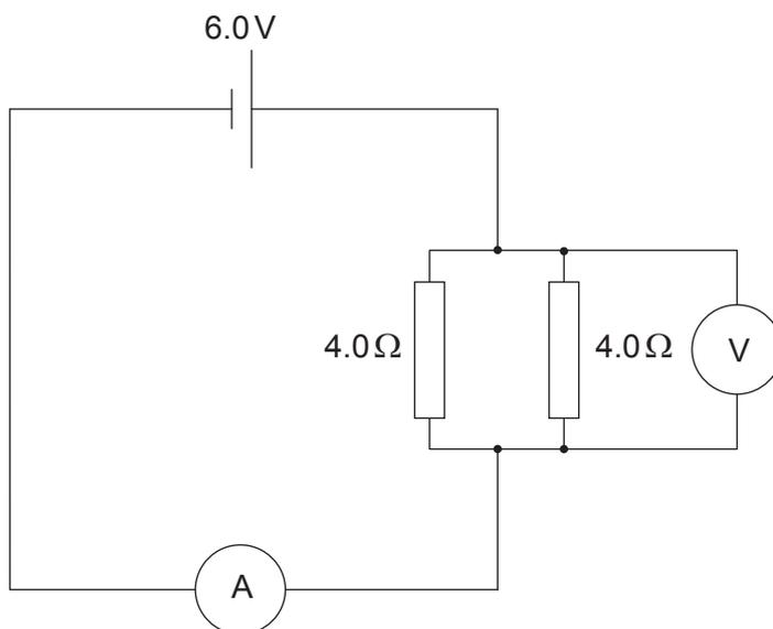
The ammeter has resistance equal to 1.0Ω and the voltmeter is ideal. What are the readings of the ammeter and the voltmeter?
