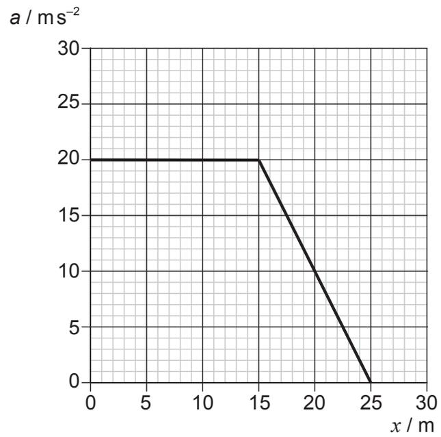
The mass of the object is 3.0 kg. What is the total work done on the object?
