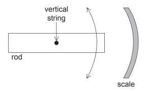
The student starts the rod oscillating and measures the largest displacement for each cycle of the oscillation on the scale and the time at which it occurs. The student begins to take measurements a few seconds after releasing the rod.
