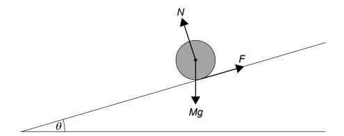
The diagram shows the three forces acting on the cylinder. N is the normal reaction force and F is the frictional force between the cylinder and the slope.
