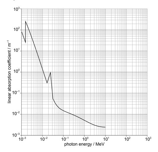
(a) X-rays are incident on an aluminium sheet of thickness 8.0 cm. Calculate the fraction of the incident X-ray intensity that emerges from this sheet for photon energies of
