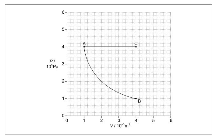
The temperature at A is 350 K. An identical mass of the same ideal monatomic gas undergoes an isobaric change from A to C.
