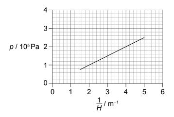
The equation of the line of best fit is  $p = a + \frac{b}{H}$ .
