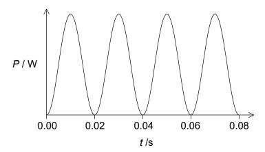
What are the frequency of the ac power supply and the average power dissipated in the resistor?
