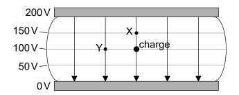
What is the work done, in nJ, by the electric field in moving a negative charge of magnitude 1 nC from the position shown to X and to Y?
