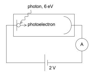
What is the maximum kinetic energy of the photoelectrons that reach the anode?
