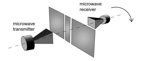
The receiver is then rotated through 180° about the horizontal dotted line passing through the microwave transmitter. Sketch a graph on the axes provided to show the variation of received intensity with rotation angle.
