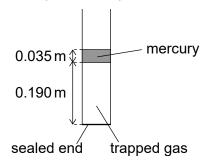
When the mercury is above the gas column the length of the gas column is 0.190 m.
