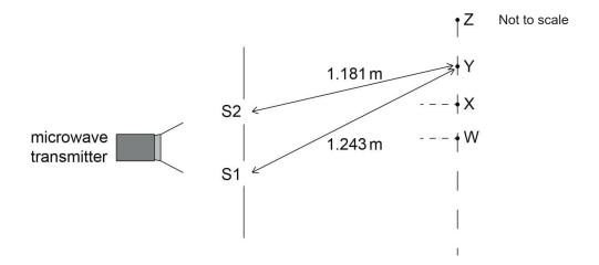
When a microwave receiver is initially placed at W which is equidistant from the slits, a maximum in intensity is observed. The receiver is then moved towards Z along a line parallel to the slits. Intensity maxima are observed at X and Y with one minimum between them. W, X and Y are consecutive maxima.
