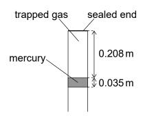
The length of the gas column is now 0.208 m. The temperature of the trapped gas does not change during the process.
