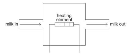
The temperature of the milk is raised from 11 °C to 84 °C. A mass of 55g of milk enters the sterilizing unit every second.
