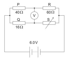
The resistance values of P, Q and R are  $40\Omega$ ,  $16\Omega$  and  $60\Omega$  respectively. The emf of the power supply is  $6.0\,\text{V}$  and its internal resistance is negligible.
