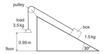
The load has a mass of 3.5 kg and is initially 0.95 m above the floor. The mass of the box is 1.5 kg.
