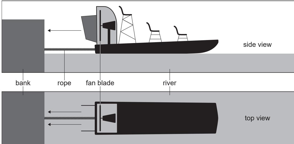
An airboat has a fan blade of radius 1.8 m. This fan can propel air with a maximum speed relative to the boat of  $20 \text{ ms}^{-1}$ . The density of air is  $1.2 \text{ kg m}^{-3}$ .
