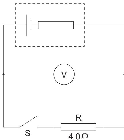
When S is open the reading on the voltmeter is 12V. When S is closed the voltmeter reads 8.0V.
