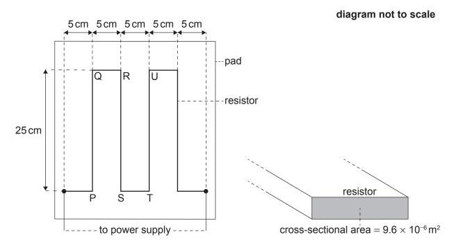
When there is a current in the resistor, the temperature in the pad changes from a room temperature of 20 °C to its operating temperature at 35 °C.
