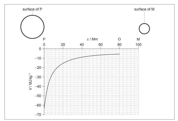
The graph shows the variation of gravitational potential V with distance x from the surface of P to O.
