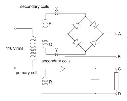
Two of the secondary coils, P and Q, are connected in series to a diode bridge. There is no load resistor between A and B.
