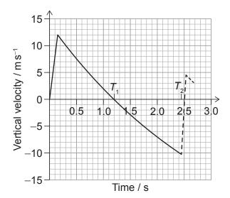
The bottle reaches its highest point at time  $T_1$  on the graph and returns to the ground at time  $T_2$ . The bottle then bounces. The motion of the bottle after the bounce is shown as a dashed line.
