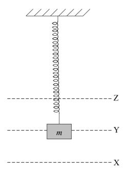
The object is pulled down to the position marked X and then released such that the object oscillates between the positions X and Z with simple harmonic motion.
