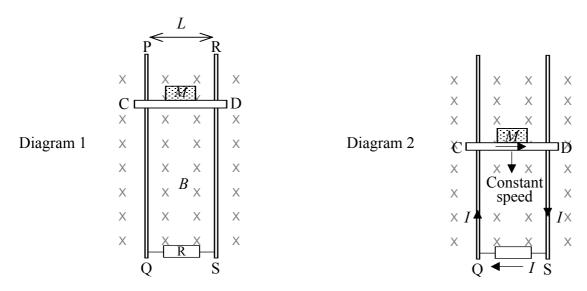
(a) Draw diagrams showing the forces acting on the loaded rod in the two cases below. Show and **label** the force(s) acting on the rod in each case.
