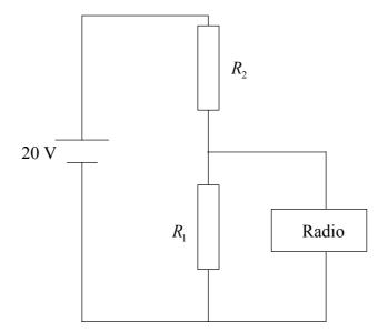
The resistances  $R_1$  and  $R_2$  are very much less than the resistance of the radio.
