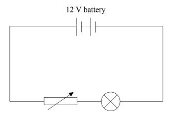
On the circuit above, add circuit symbols showing the correct positions of an ideal ammeter (a) and an ideal voltmeter that would allow the *V-I* characteristics of this lamp to be measured. [2]
