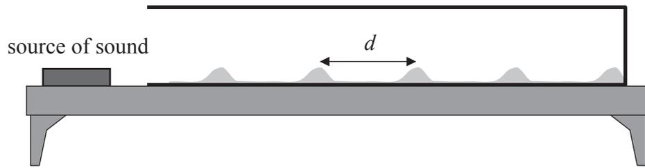
The distance between two consecutive piles of powder is  $d$  and the speed of sound in the tube is  $v$ . The frequency of the source is
