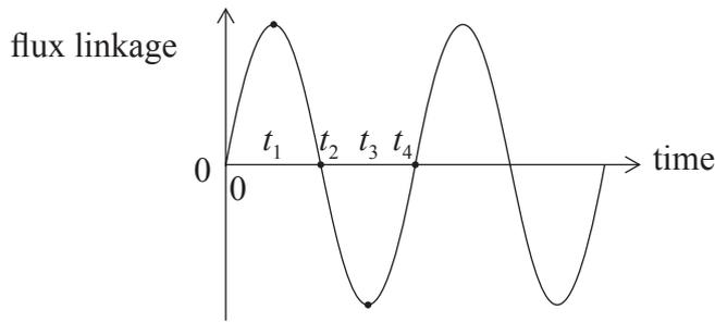
At which times is the induced e.m.f. equal to zero?
