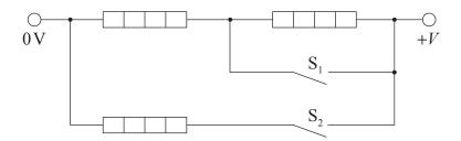
Each heating element dissipates power P when connected to a supply of V volts. The resistance of each element may be considered to be constant.
