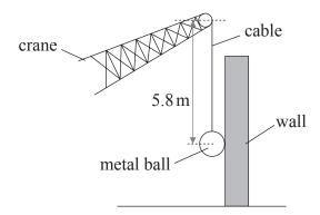
In order to knock down a wall, the metal ball of mass  $350 \,\mathrm{kg}$  is pulled away from the wall and then released. The crane does not move. The graph below shows the variation with time t of the speed v of the ball after release.
