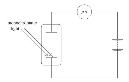
The metal surface has work function 2.4 eV and the threshold wavelength for light incident on the surface is  $\lambda_s$ . The current in the photo-cell is measured using a microammeter.
