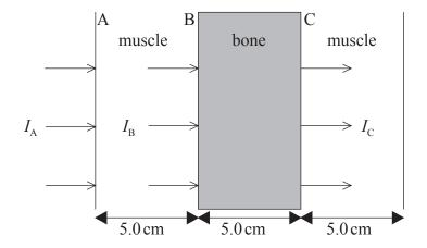
The intensity of the X-ray beam at the surface A of the leg is  $I_A$ . At the surface B of the bone, the intensity is  $I_B$  and the intensity of the beam emerging at surface C of the bone is  $I_C$ .
