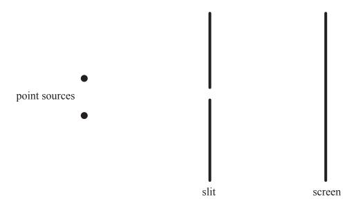
The images of the two sources on the screen are just resolved according to the Rayleigh criterion.
