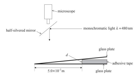
A beam of monochromatic light is incident on the wedge film. The light that is reflected at right angles to the wedge, is viewed using the microscope. A system of parallel fringes of equal spacing is observed in the field of view of the microscope.
