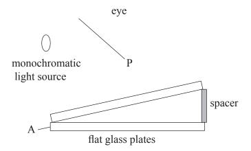
It is arranged for light from a monochromatic source to be incident on the plates by reflection from another glass plate P. The light reflected from the wedge is viewed from above as shown in the diagram. A system of equally spaced, parallel fringes is observed. (The diagram is not to scale.)
