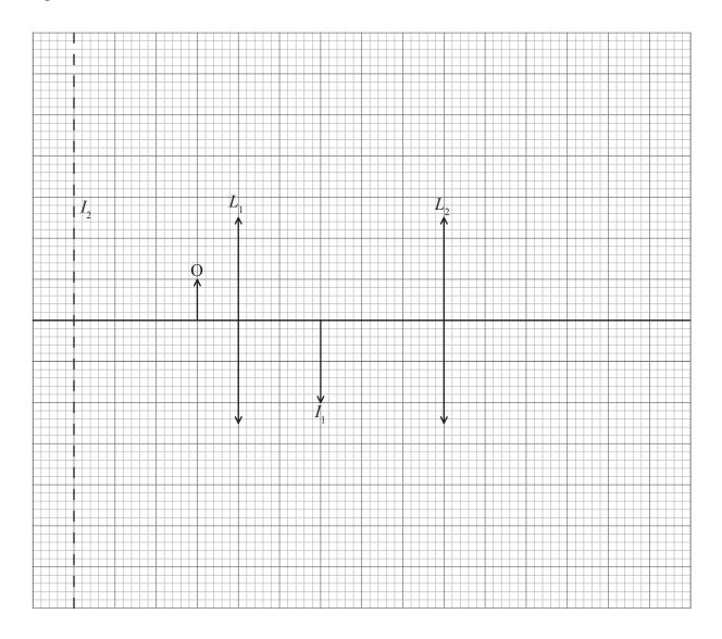
$I_1$  is the image of the object O formed by the objective lens  $L_1$ . The final image formed is in the plane shown by the dotted line labelled  $I_2$ .
