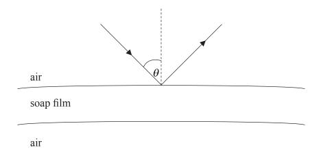
Constructive interference takes place for light of wavelength  $\lambda$  at the angle  $\theta$ .
