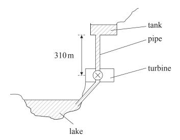
Water stored in the tank is allowed to fall through a pipe to a lake via a turbine. The turbine is connected to an electrical generator. The pumped-storage ac generator system is reversible so that water can be pumped from the lake to the tank.
