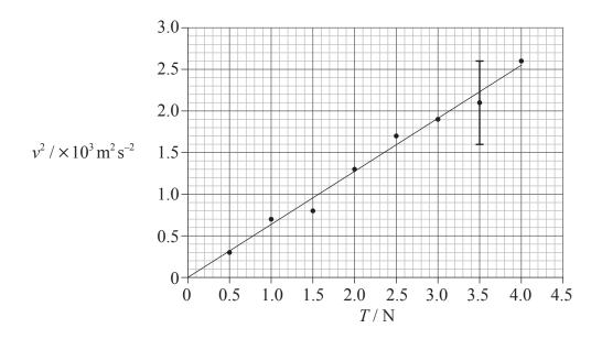
The best-fit line shown takes into account the uncertainties for each data point. The uncertainty in  $v^2$  for T=3.5 N is shown as an error bar on the graph.
