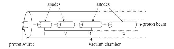
The vacuum chamber contains a succession of cylindrical anodes of which only four are shown, anodes 1, 2, 3 and 4.
