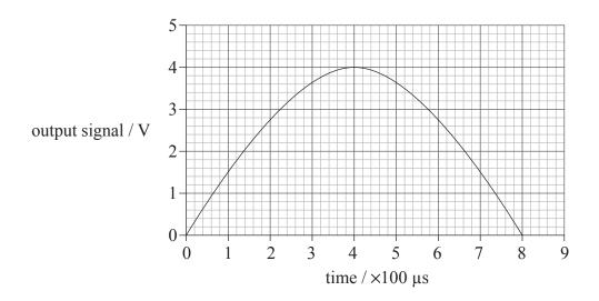
In order to convert the analogue signal into a 3-bit digital signal it is sampled every  $100\,\mu s$ . The possible output voltages of the analogue to digital converter that is used are shown below.
