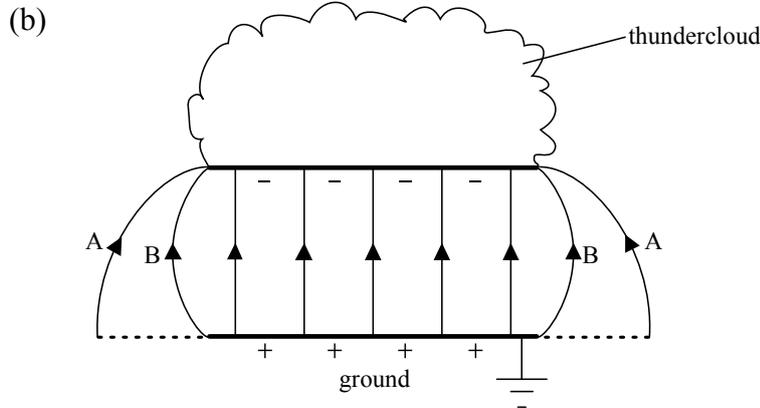
lines connecting plate and ground equally spaced in the central region of thundercloud
