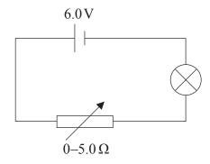
Explain, with a calculation, why this circuit will not allow for a full range of potential difference from 0V to 6V across the bulb. Assume that the resistance of the lamp remains constant at a value of  $2.4 \Omega$ .
