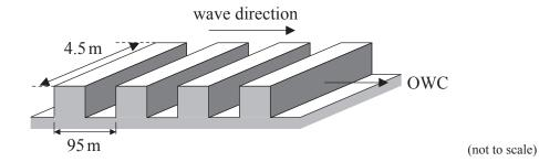
Assuming that the waves have a rectangular cross-section, determine the minimum wave amplitude that will be required in order for the OWC to produce a power output of 0.10 MW.
