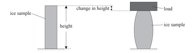
After the load has been applied, it is observed to move downwards at a constant speed v as the ice deforms. The constant speed v is measured for different loads. The graph shows the variation of v with load W for a number of identical samples of ice.
