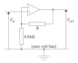
The overall gain of this circuit is  $\frac{V_{\text{OUT}}}{V_{\text{IN}}} = 26$ . Calculate the resistance of resistor *R*. [2]
