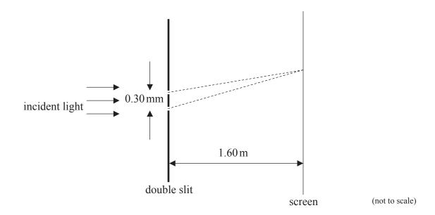
Calculate the fringe spacing on the screen.
