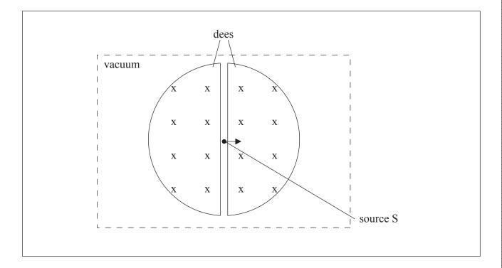
Protons are injected into the cyclotron from a source S. The arrow indicates the direction of a proton after it has left the source. The magnetic field is directed into the plane of the page.
