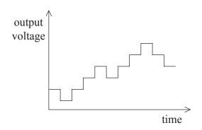
State and explain **two** ways in which the output signal could be made to be a more accurate reproduction of the input signal.
