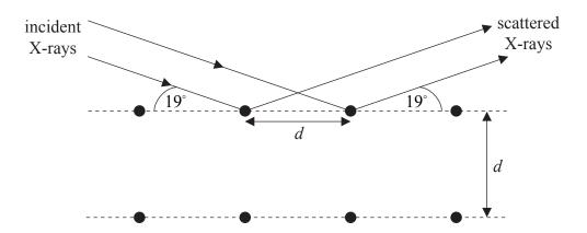
Calculate the lattice spacing *d* of these planes.
