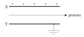
A uniform magnetic field also exists in the region between the plates. The direction of the field is such that the protons pass between the plates without deflection.
