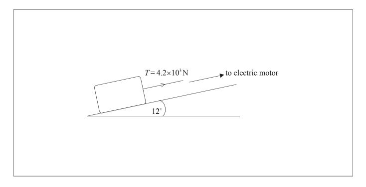
The incline makes an angle of  $12^{\circ}$  with the horizontal. The weight of the block is  $1.5 \times 10^{4}$  N and the tension *T* in the cable is  $4.2 \times 10^{3}$  N.
